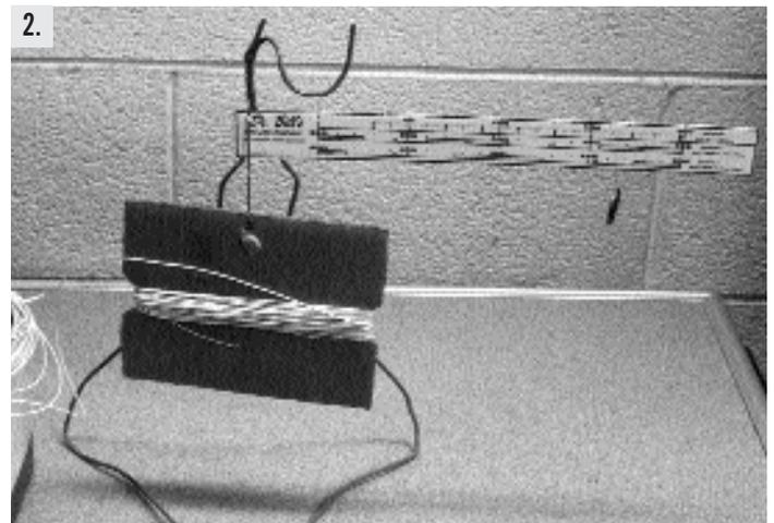
A small dab of "stick putty" is used to zero the scale before use. Line is measured and wrapped around the slotted cardboard as shown, or you can size the card perfectly so that each wrap equates to a certain length of line (see text).
