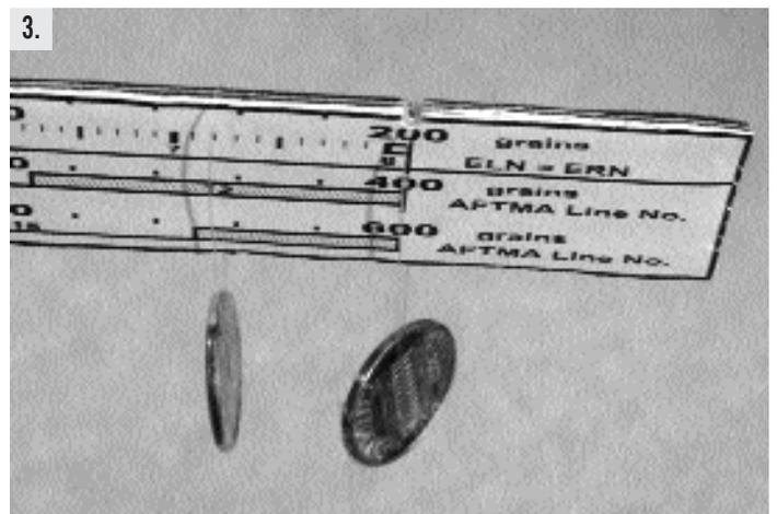
As you move to more or heavier line, you'll need to place a cent into the notch at the 200 grain line and then use another cent to slide on the beam until balance is achieved. With a cent or cents located in the notch, make sure to take your measurement reading from the correct line.
