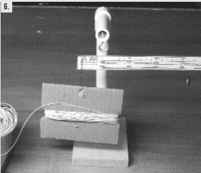
Notice that we have located the remainder of the line not being weighed onto a box so that it is not adding any weight or influence to that length which we are attempting to weigh. Position the line not being weighed in such a manner so that it does not influence your results.
