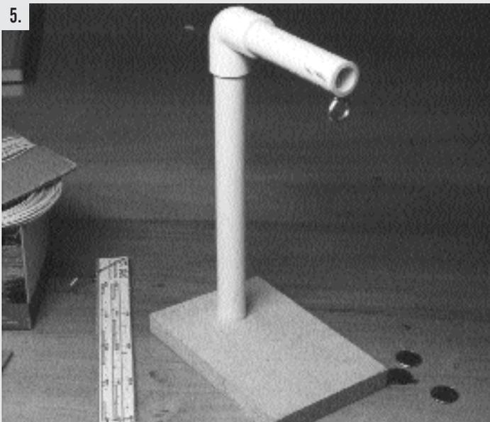
If you plan on measuring many lines, you may desire a sturdier stand from which to hang your beam scale. This one has been fabricated from some small diameter PVC pieces and a wooden base. The make up of your stand is really not all that important. Just make sure the beam scale can move freely.
